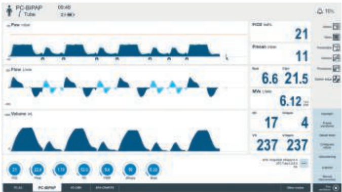
Fig. 1 PC-BIPAP with mandatory and spontaneous mechanical breaths
