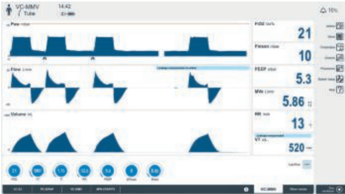
Fig. 2 VC-MMV/AutoFlow with mandatory breath and spontaneous breathing
